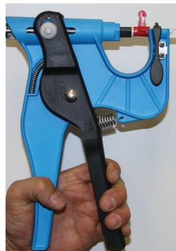
④ Carefully squeeze the applicator handles together, guiding the punch tip into place if necessary. When fully seated the gun bolt will rest flush against the red plastic clip.
