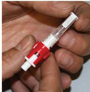
② Ensure the tube retainer at the base of the applicator gun is open. Push the retainer clip to open.
