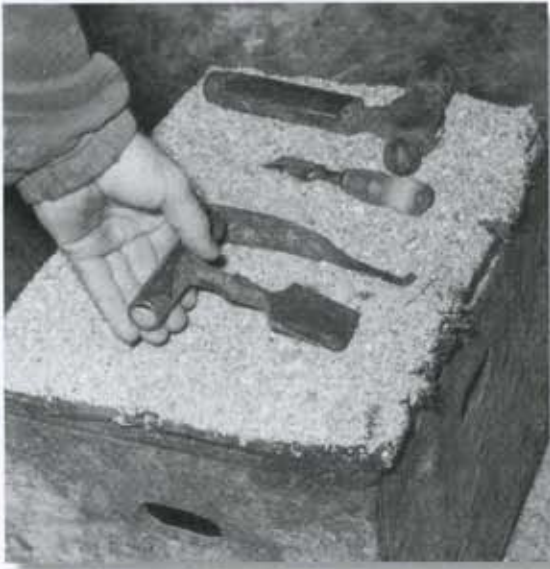
Tools used for trimming feet include (bottom to top) a 2-inch chisel with T-bar; hoof knife; 1-inch chisel and hammer.
