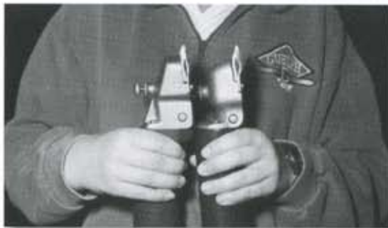
Note the special plucking blades on the right, compared to the regular clipping blades on the left.
