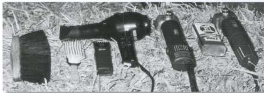
Equipment used by an advanced clipper includes (l to r) soft, long-bristled brush; small topline brush; rechargeable clippers; powerful hair blower; large animal clippers with Aesculap plucking blades; three-in-one clipper oil; large animal clippers with normal Stewart blades.
